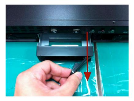
Pull the HDD tray out of the case.
